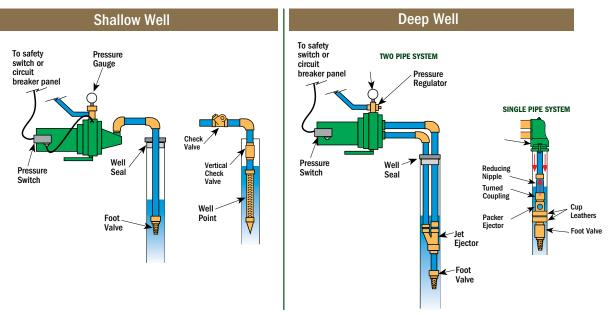
For a jet nozzle to be effective it must be combined with a venturi. The venturi changes the high-speed jet stream back to a high-pressure for delivery to the centrifugal pump. The jet and venturi are simple in appearance but they have to be well engineered and carefully matched to be efficient for various pumping conditions. The jet nozzle and venturi are also known as ejectors/ejector kits.
