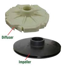
The head or pressure that a pump will develop is in direct relation to the impeller diameter, the number of impellers, the eye or inlet opening size, and how much velocity is developed from the speed of the shaft
